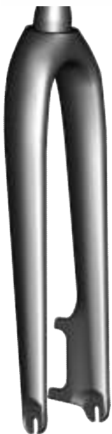
CF 56 配车架C0S132 FORKS: For 700C wheel MATERIAL :100% carbon Carbon drop out WEIGHTS:570±10g
